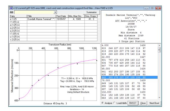
Data files in the working directory are listed under the data item in the grid. The program recognizes most common FWD file formats, including one EXCEL spreadsheet format. Initially, all other information items are blank. Hitting the Summarize button fills in this information. This summary can be saved to the hard disk. The data is stored in the file data.dds and is illustrated below.
