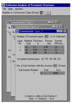
The pavement construction information can be defined for various lengths of the pavement by reference to the station numbers. In the example given, three construction types have been defined for the FWD data file. The user must define a length of pavement associated with each construction type.
