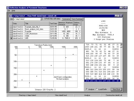
Single data points can be analyzed by interactively clicking on a deflection bowl (providing a CDT file has been made). Information displayed on the deflection bowl graph includes the layer stiffness and the calculated stiffness for each pavement layer. The thickness of the soil layer is the calculated thickness to an assumed rock foundation. The statistic RMSerr/Max
