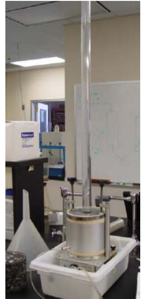
Water permeability apparatus (Mallick and Bergendahl, 2004)
