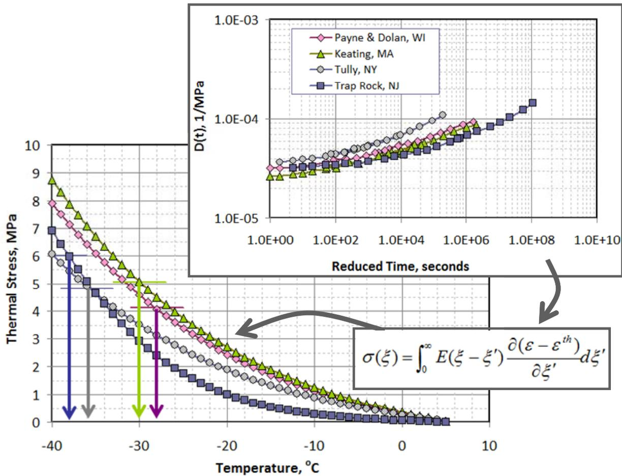
**FIGURE 5** Creep compliance data (at  $T_{ref} = -40^{\circ}\text{C}$ ) obtained from core and gyratory compacted specimens (top right) used to compute estimated thermal stress (bottom left) for various mixes (horizontal lines in bottom left represent tensile strength evaluated at  $-30^{\circ}\text{C}$ )
