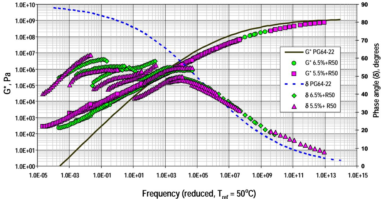
Modified materials denoted by 5.5%+R50 and 6.5%+R50. The 5.5 and 6.5 refer to the binder content (PG64-22) in the unmodified mixture. A 6.5% blend with R50 (added at a 2.25%/45lb per ton level) results in a PMM concentration of 25.7% of the total binder.
